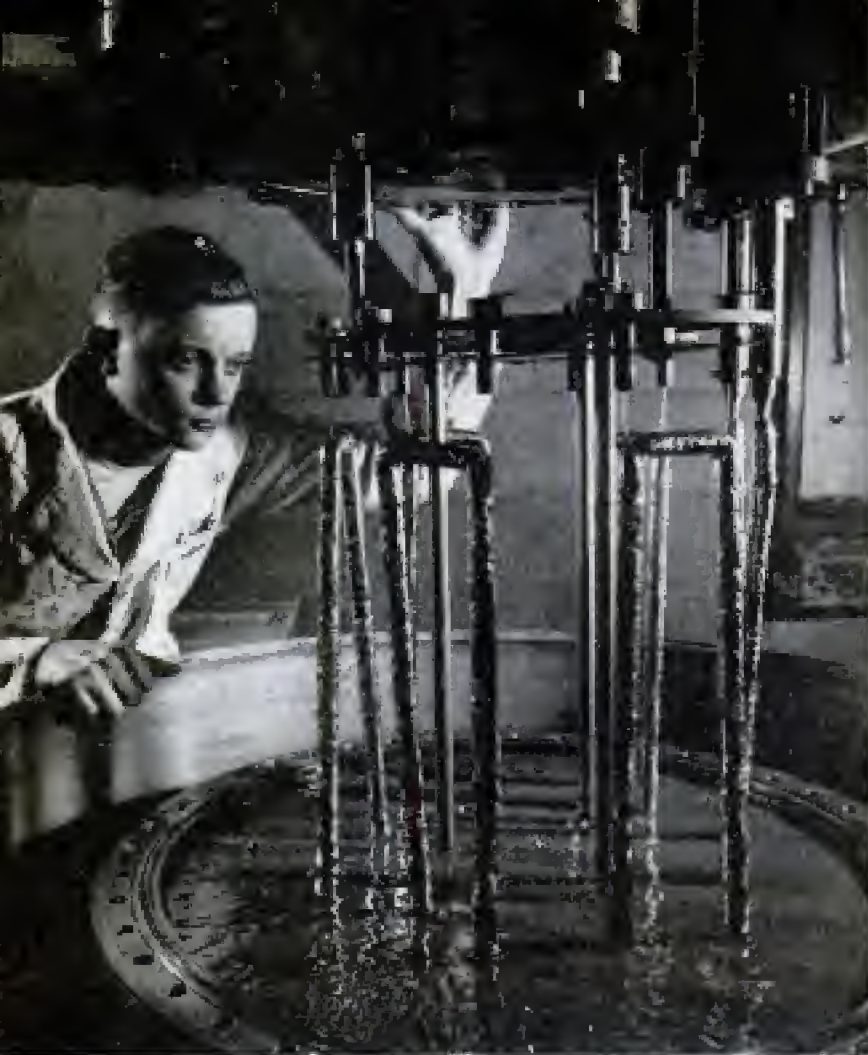
Glistening bars of zirconium, 99.9 percent pure, are raised from tank which has been flooded with water as a precaution against fire. Metal is deposited on wires by electrochemical action. Below, ingots of zirconium being tested for hardness before production use at Westinghouse Atomic Power Division
